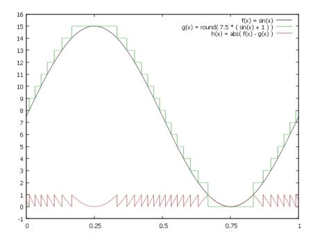
The black line shows the original, (time and value) continuous signal. The green line shows the original signal after quantization to a value range from 0 to 15, representing a 4bit integer.
