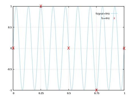
Time-continuous signals with different frequencies can obviously result in the same time-discrete signal when using the same sampling frequency.
