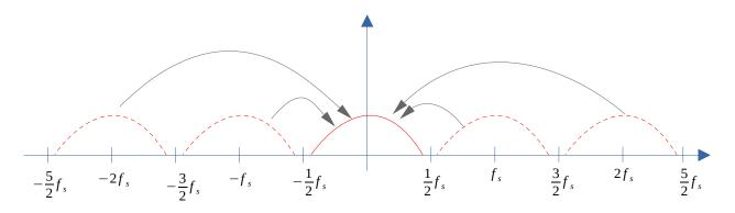
The frequency spectrum becomes periodic, i.e. adding a whole multiple of the sampling frequency  $f_s$  to the signal frequency  $f_{sianal}$  results in the same time-discrete signal. Or in mathematical terms:
