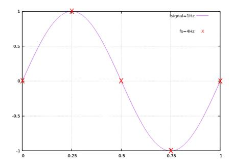
These four samples are sufficient to reconstruct the original, time-continuous signal.
